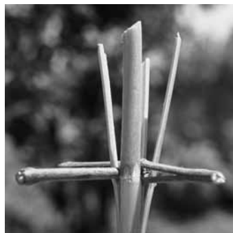
Fig. 2 The tool ( yıldız yargeç ) made of two twigs of Vitex is used for splitting cane ( Arundo donax ). Bodrum 2000 (F. Ertuğ).
