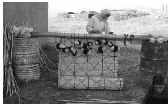
Fig. 10 A reed screen weaving with a "loom" with 18 stone weights. Cizre-Şırnak 2006 (Adnan Gençay).
